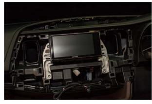
Make all connections to the Kenwood head unit and mount the head unit to the factory mounting locations.
