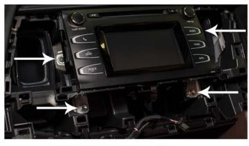
Unscrew the 4 (10mm) bolts and remove the head unit.
