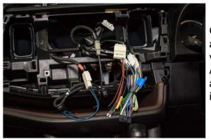
Connect the Kenwood harness and antenna adapter to the vehicles connectors.
