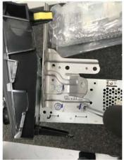
Remove the brackets from the factory head unit and panel clips to re-use.
