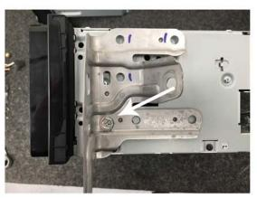
Re-install the factory brackets onto the Kenwood head unit in the position shown.
