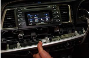
Un-clip and remove the climate control with the panel it is attached to.
