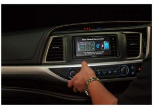
Attached the factory clips to the BKTO093 and clip into place. Then re-install everything in the reverse order to complete installation.
