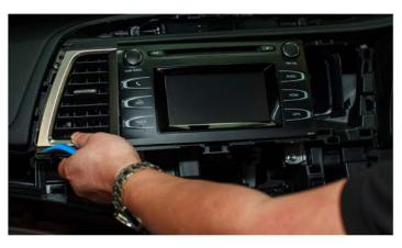
Un-clip and remove the air vents on either side of the head unit.
