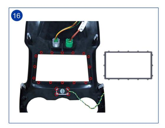
Place the speaker onto the Connects2 fascia and with a soldering iron, melt the four plastic tabs (highlighted in the picture) in the corner of the speaker.
