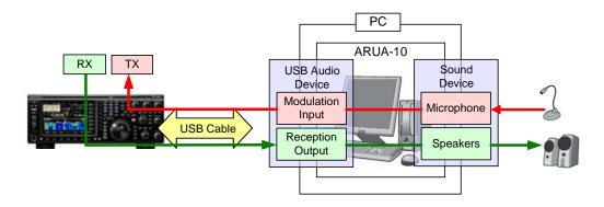
Diagram 2.1: Operation Using the USB Audio Function
